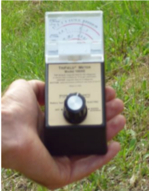
Fig.1 Outside of Om Shree Dham property on the public road under power lines the meter registers quite high EMF. On low sensitivity setting.
